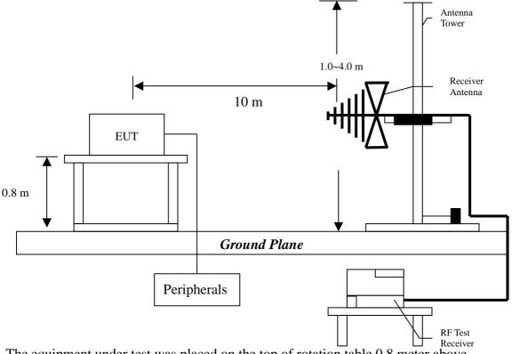
The equipment under test was placed on the top of rotation table 0.8 meter above ground plane.
