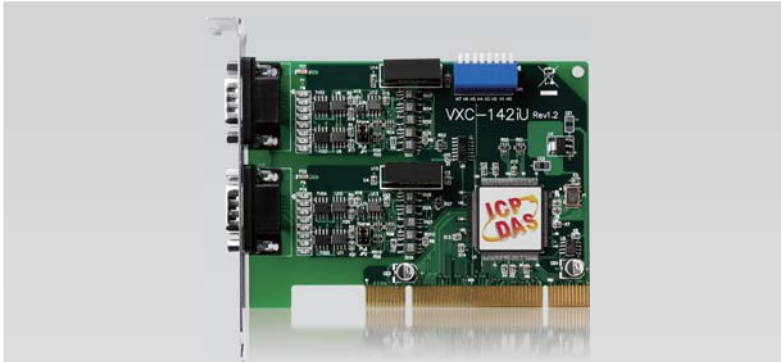
VXC-112AU / VXC-112iAU / VXC-142AU / VXC-142iAU Universal PCI, 2-Port RS-232 or RS-422/485 Communication Board
