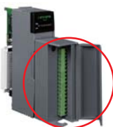
I-87018PW-G/S CR= I-87018PW connects CN-1824 directly
