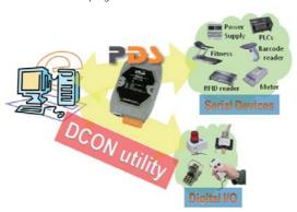
"Virtual I/O" is the extension of "Virtual COM" technology that simulates PDS's digital I/Os control as a virtual COM port (Port I/O) application on PC. And since now, you are able to access PDS's digital DCON protocol through the virtual COM port. Besides, DCON utility also supports configuring PDS's digital I/Os through the help of "Virtual I/O" technology. So you can diagnose PDS's digital I/Os and complete the I/Os application in a convenient way.
