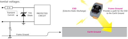
Under normal operating conditions, the TVS diode presents high impedance (appears as an open circuit) to the protected component. If the voltage exceeds the limitation, the TVS diode avalanches, providing a low impedance path for the transient current. As a result, the transient current is diverted away from the protected components and shunted through the TVS diode. The device returns to a high impedance state after the transient threat has passed.
