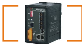
RSM-405FCS Single-mode Fiber Redundant Ring Switch
